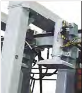
Cylinders and pressure clamps fitted with independent open/close valve.
