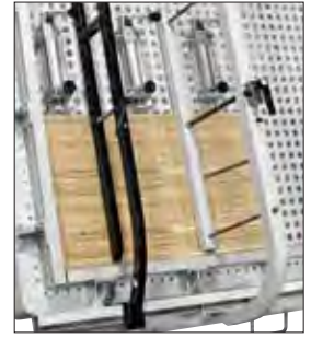
Fixed and sliding front clamp.
