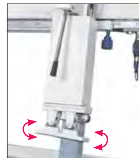
Pivoting thrust feet for tilted frames.
